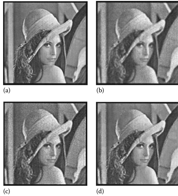
FIGURE 25.4 (a) Original image, (b) degraded image at 25 dB SNR, (c) restored image using Kaczmarz iterations, and (d) restored image using the modified Kaczmarz algorithm in a POCS framework. (Courtesy of IEEE: Kuo, S.S. and Mammone, R.J., IEEE Trans. Signal Process. , 40, 159, 1992.)
